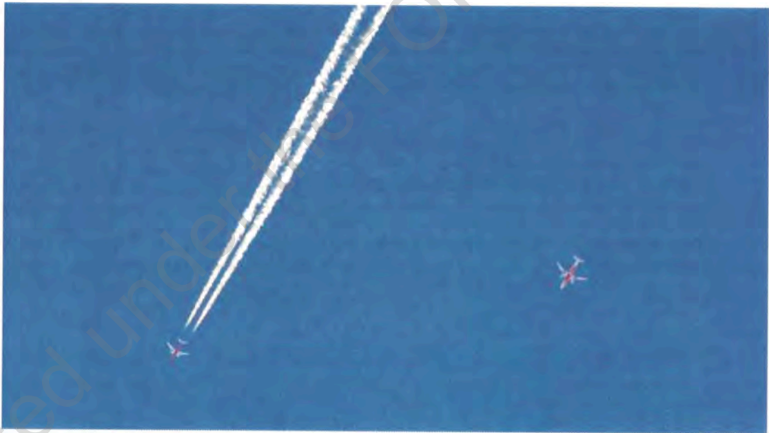
Above: Figure depicts two aircraft on the same track, at different altitudes, one creating a condensation trail and the other not. Highlighting that the atmospheric conditions create the condensation trail.
